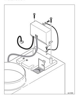
The control module must be installed above the cooker hood housing.
